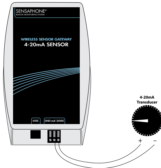
4-20mA Transducer using 24VDC power supply
